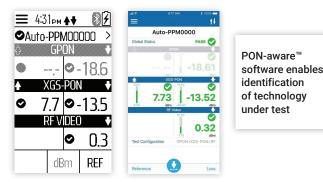
Optical Explorer (OX1) to validate expected downstream power value and identify causes of failure on the spot. As the service is active, an out-of-band wavelength (1650 nm) on a filtered port must be used so as not
